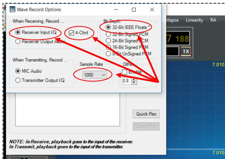
This configures the recording of antenna signals in a WAV-format that resembles a 4-channel audio file, but contains:
