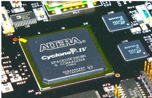
The ANAN-100D is the first HF transceiver with a true phase coherent dual front end comprising of two 16 bit 130MSPS ADCs and a large Cyclone IV FPGA which allows for a huge amount of headroom and DSP processing power, the current
