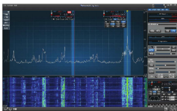
SmartSDR screen - panadapter + waterfall with 2 slice receivers. Horizontal lines on waterfall are local electric fence ticks.
