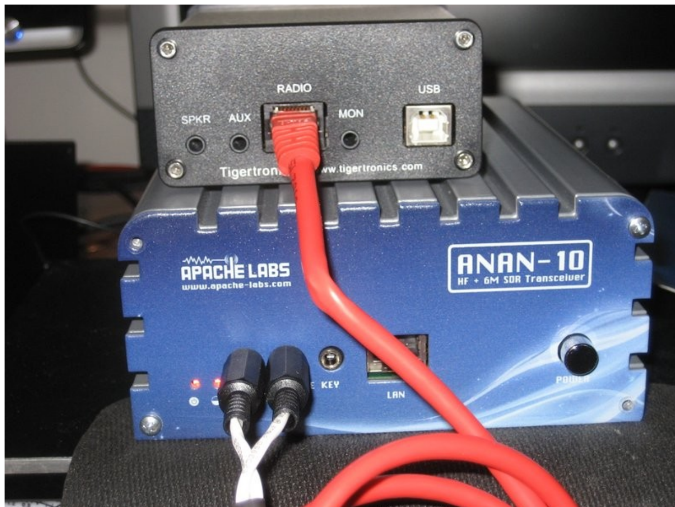
Completed SignalLink USB to Hermes/ANAN-10 Cable
